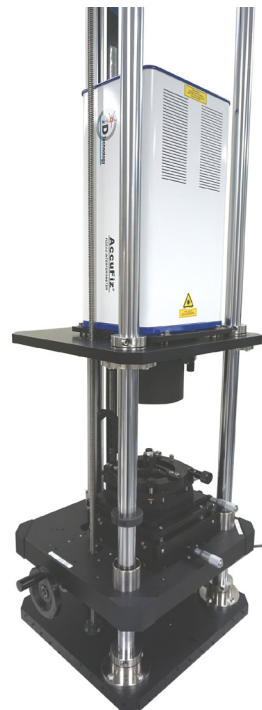
Figure 7. A Fizeau interferometer in a look-down configuration with a precision positioning stand.
