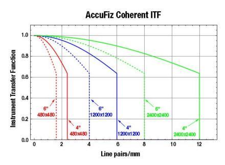
Figure 5. Instrument Transfer Function (ITF) for various AccuFiz models. The ITF is equivalent to the normalized instrument response as a function of spatial frequency (decreasing spatial period).
