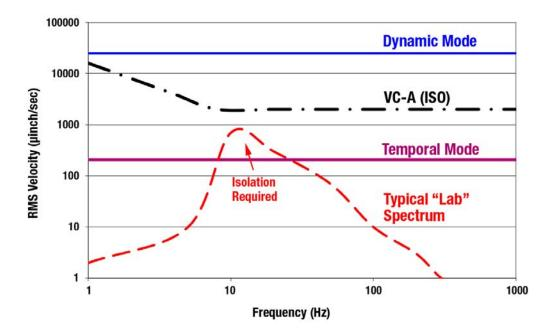
Figure 3. AccuFiz response to vibration. Dynamic mode functions in virtually any environment, whereas temporal mode requires isolation even in typical lab settings.
