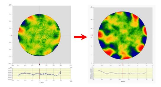
Figure 9. Typical artifact suppression due to dust on an optic.
