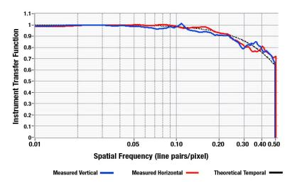
Figure 6. Measured ITF for a production 100mm aperture, 1.44MP AccuFiz. Dotted line is the theoretical maximum (detector-limited response).
