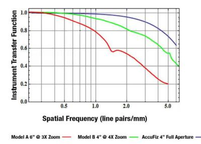
Figure 7. Comparison of a 4" aperture AccuFiz at full aperture vs other models of interferometers while zoomed.
